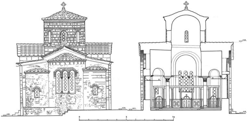
Figure 208 Katholikon of the Petraki monastery. Elevation of the east side and north–south section. Actual state. Drawing by P. Koufopoulos and M. Myriantheus.
